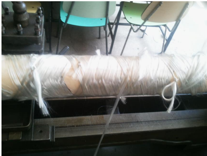
Fig. 6 – Composite material wrapped around the template
